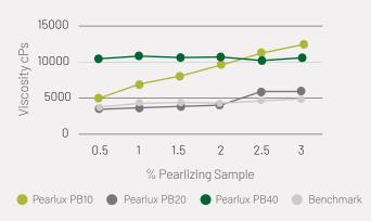
The viscosity of the system increases as the amount of Pearlux PB10, Pearlux PB20 and Benchmark increases. Pearlux PB10 has the highest viscosity among the three samples.
